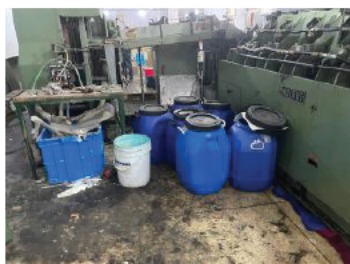
No secondary container for chemical (3).JPG
