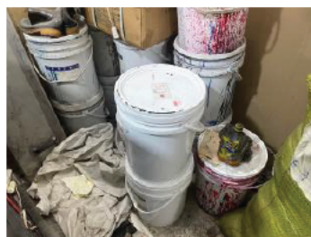
No secondary container for chemical (1).JPG
