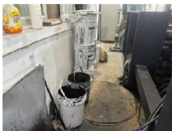
No secondary container for chemical (2).JPG
